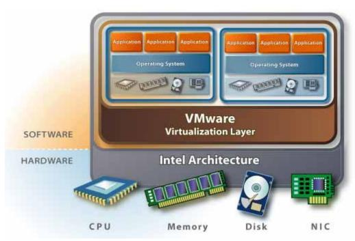
The VMware virtualization layer sites between the hardware and software and allows users to create virtual machines that are the full equivalent of a standard x86 machine
