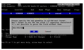
4. You can now enter the correct geometry of 261 cylinders, 255 heads and 63 sectors per head by typing 261/255/63 in the dialog box. Then click **OK** and continue installing FreeBSD.
